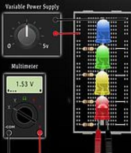
The threshold voltage ( $V_t$ ) of an LED is the amount of voltage required to make the LED start producing photons. To convert the measured threshold voltage to energy, we multiply by the elementary charge constant ( $e = 1.602 \times 10^{-19}$ ):
